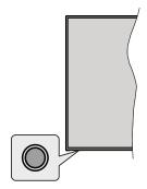
The control button allows you to control the Quick Standby-On functions of the TV.
