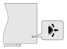
The control switch allows you to control the Programme and Quick Standby-On functions of the TV.
